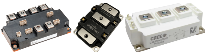
Fig. 8. Selected SiC MOSFET power modules. From left: Mitsubishi Electric FMF300BX-24A, Wolfspeed CAB400M12XM3, Cree CAS300M12BM2
