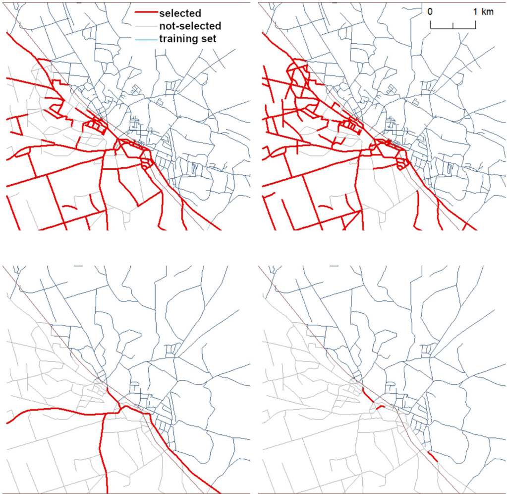
Fig. 7. The results for the road sections obtained by the RST method in the area of Chocianów: on the left – the CN2 algorithm, on the right – the LEM2 algorithm; at the top – 10k→50k selection, at the bottom – 50k→250k selection; the selected objects are marked in red (source: A. Fiedukowicz 2017)
