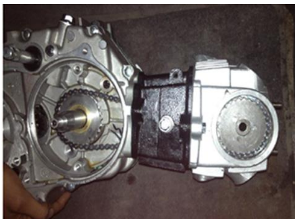
Fig. 3. Crankshaft and camshaft assembly
