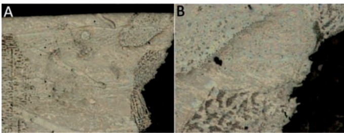
Fig. 7. Microscopic images of fractures of laser-welded samples. Sample cross-section at the fracture site A – magn. x 50, B – magn. x 200
