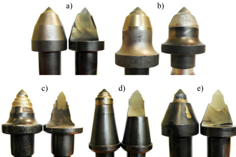
Fig. 6. Options of additional protection of the tangential-rotary picks against abrasive wear (Sandvik, 2013) a) standard pick, b) welded picks, c) pick with ring made of sintered carbide, d) pick with two rings made of sintered carbide, e) pick with lowered body and sintered carbide of the type CAP
