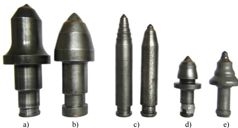
Fig. 5. Tangential-rotary picks used for: a) longwall shearers, b) roadheaders, c) shearers used for salt mining, d) milling machines for concrete cutting, e) milling machines for asphalt cutting
