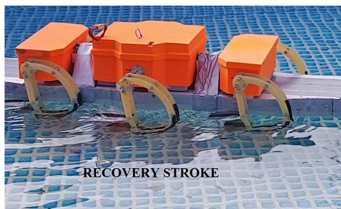
Fig. 11. Amphibious locomotion. The above figure shows the experimental setup for FLHex in water-surface test with A = 50^\circ , A_0 = 20^\circ , f = 0.5 Hz (Eq. (4))
