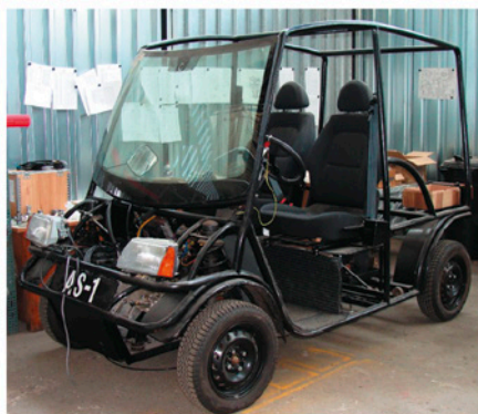
Fig. 24. Vehicle prototype, to be used as a base for the installation of the control system units having been developed (MCU, BMS, GBCS)
