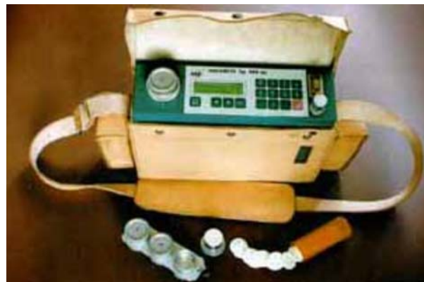
Fig. 3. Mining radiometer RGR-40. The radiometer measures alpha potential energy concentration of radon daughters and concentration of RaA (Po-218), RaB (Pb-214), and RaC+RaC' (Bi-214+Po-214).
