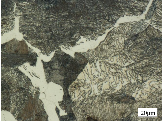
Fig. 3. Counter-specimen microstructure after normalizing: pearlite, ferrite, non-metallic inclusions
