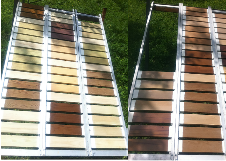
Fig. 1. The control and test samples before weathering in the Uzungöl plateau
