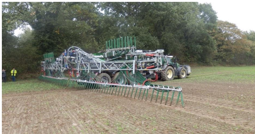
Figure 2. Use of the field set for spreading acidified slurry on the field with trailing hoses.
