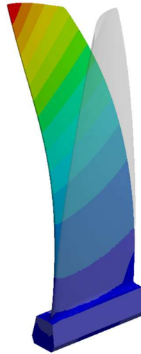
Fig. 2. Modal analysis of a blade
