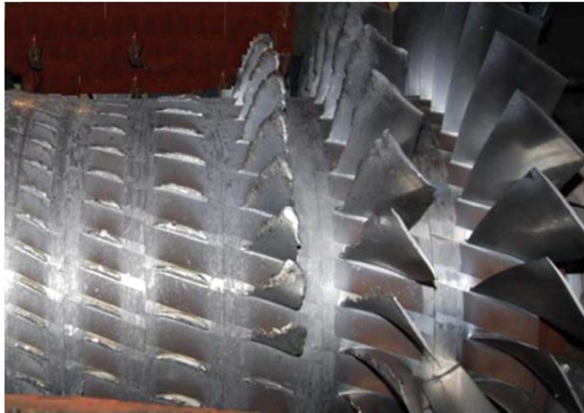
Fig. 1. View of the compressor rotor with damaged blades (FOD)
