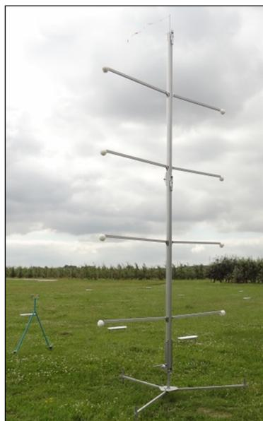
Figure 2. Airborne drift collectors on mast
