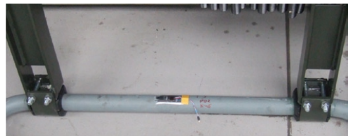
Fig. 5. Stabilizer with glued-on strain gauge
