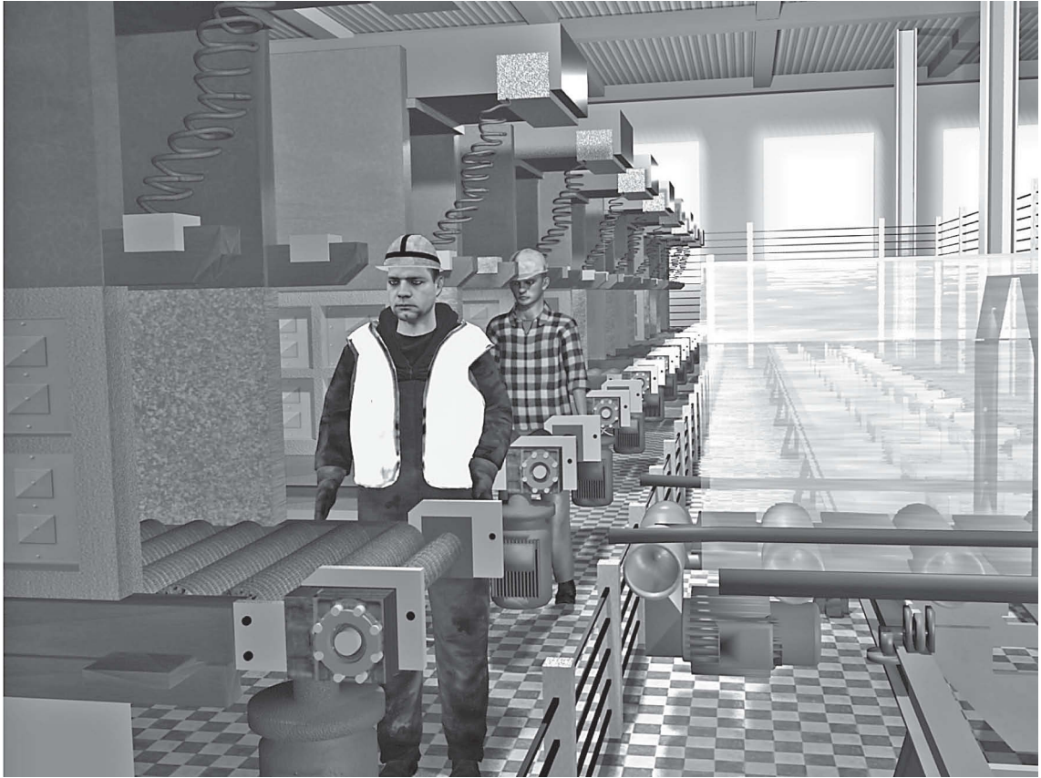
Figure 6. Virtual model of an actual assembly line used to test a vision based protective device (VBPD).
