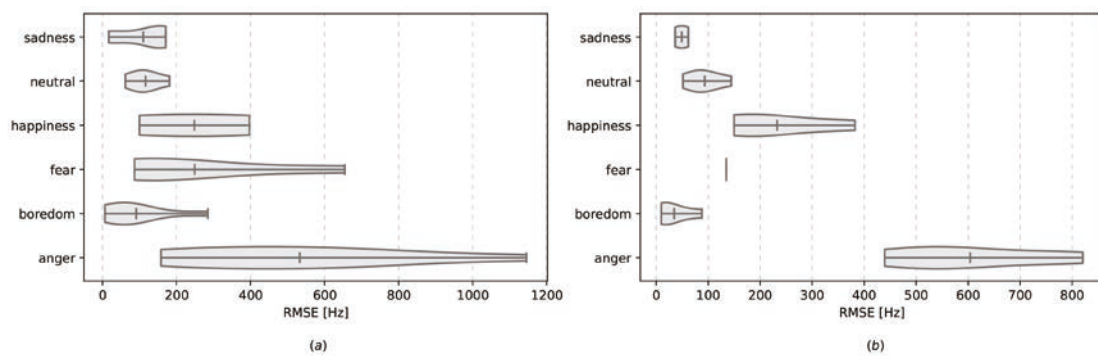
Figure 12. RMSE values for all recordings between F_0 and \bar{c} in data set: females (a), and males (b).
