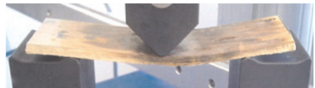
Fig. 7. 3-Point bending test of WCPC specimen in accordance with DIN EN 310 (1993)
