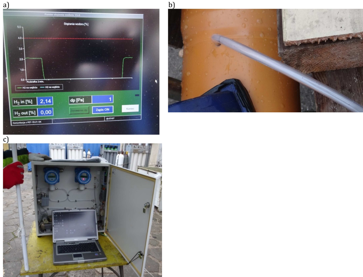
Fig. 10. The examination of the procedure of mixing hydrogen with air: a) measurement results presentation; b) sampling method; c) view of the measurement station.
