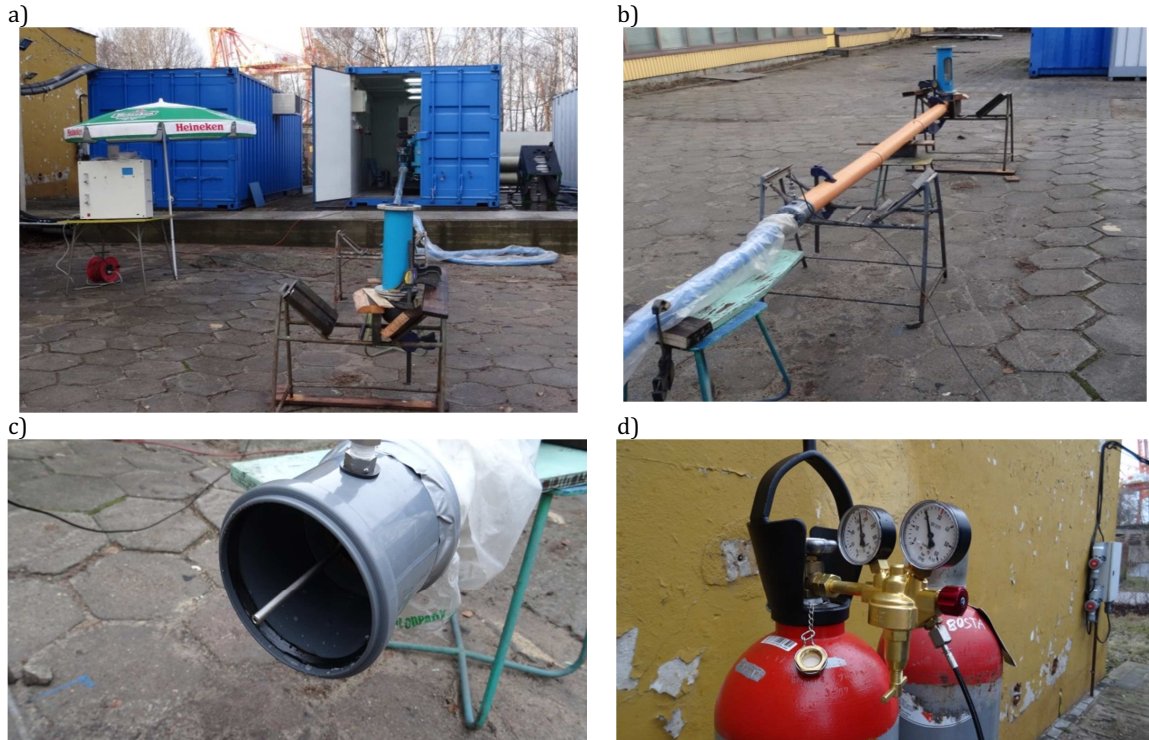
Fig. 9. A Tubular reactor for the production of a hydrogen-air mix: a) view of the air pump station located in the container, the rotametric measurement station is visible from the front; the station of hydrogen content measurement in the air is on the left; b) view of the pipe mixer; the connection of the pumping hose to the dosing head of the tubular reactor is visible closer to the reactor's inlet; c) view of the hydrogen line connection and hydrogen dosing tube to the tubular reactor; inside the hidden casing of the dosing nozzle; d) pressure regulator on the hydrogen supply .
