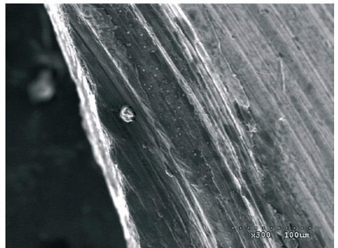
Fig. 15. Photograph of the surface of the seat in the anodized plate, mag. x70. Scratches formed during implantation of the component are marked in the photograph
