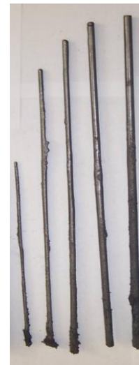
Fig. 4. The rods of fluidity test of spheroidal graphite iron, pouring temperature 1591 K (1318 0 C)
