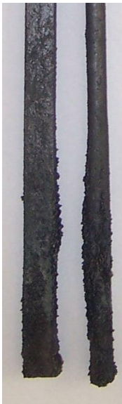
Fig. 6. The rods of fluidity test of spheroidal graphite iron, pouring of temperature ( 1313^{\circ}\text{C} ) 1586 K
