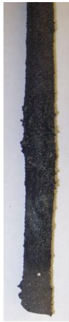
Fig. 5. The rods ( \phi 6 mm) of fluidity test of spheroidal graphite iron, pouring temperature 1591 K ( 1318^{\circ}\text{C} )
