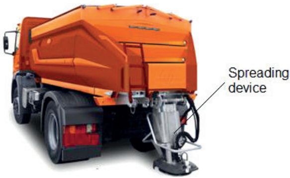
Fig. 1. Road spreading vehicle.
