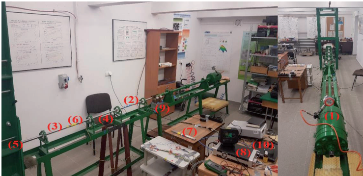
Fig. 3. SHPB test stand. Mechanical part of the station: (1) - pneumatic cannon with a barrel of loading bar-projectile, (2) - initiating measuring bar, (3) - transmitting measuring bar, (4) - soil sample in the casing, (5) - damper. Measuring part: (6) - strain gauges, (7) - compensating strain gauges, (8) - measuring device with digital memory, (9) - laser timekeeping system, (10) - computer software.
