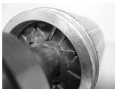
Fig. 2. Rotor and its cross-section of single-phase line start permanent magnet synchronous motor with W shape permanent magnet arrangement
