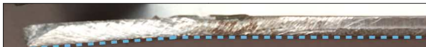
Fig. 11. Segment of adhesive joint (adherend) after destructive test. The permanent deformation of sheet is visible
