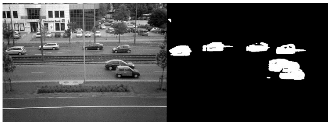
Fig. 2. Sample output of average median algorithm. Currently processed frame on the left, and the foreground on the right
