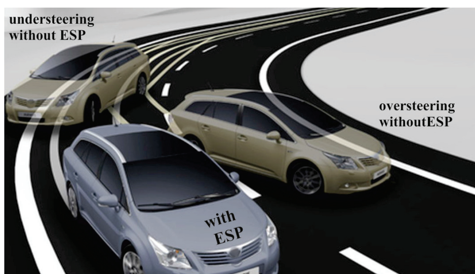
Fig. 1. Operation of ESP (electronic stability program) [3]
