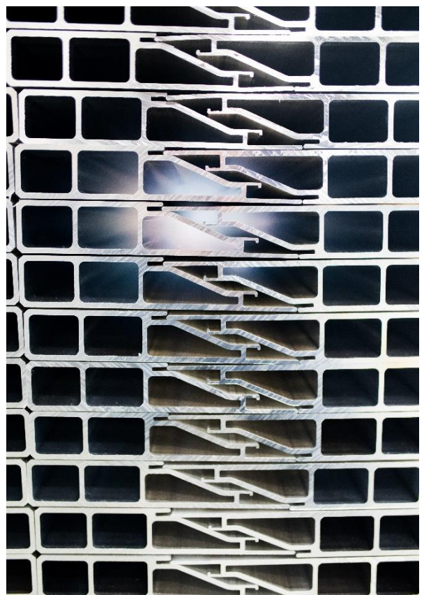
Fig. 3. Exemplary pictures of profiles from which the window and door structure of aluminum alloy 6060 is made.
