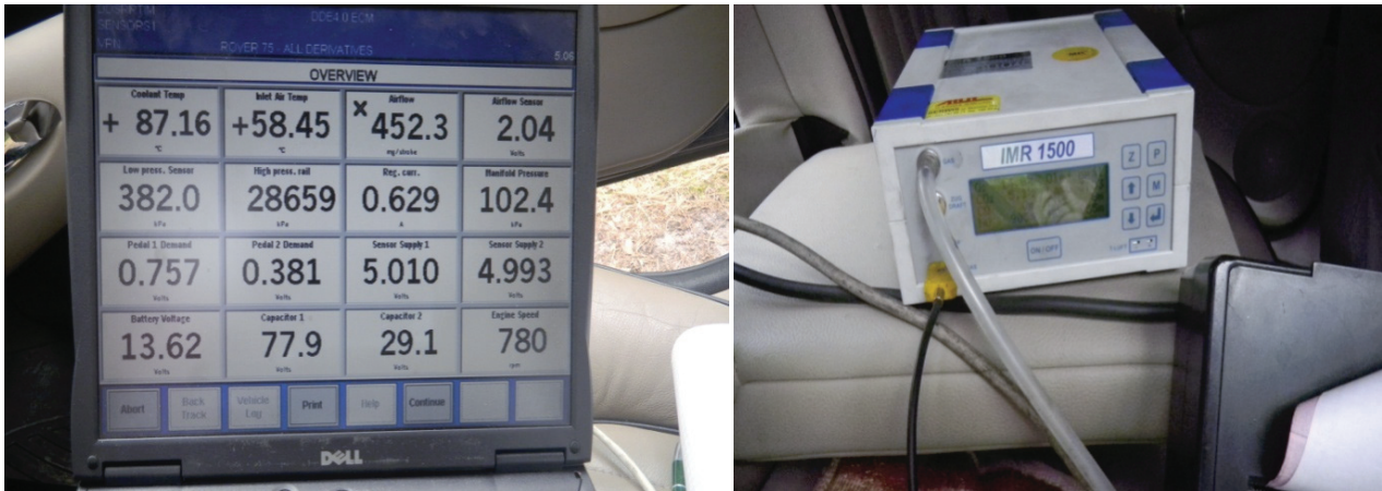
Fig. 2 Read of the controller data via TestBook T4 and IMR 1500 exhaust gas analyser
