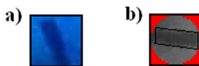
Fig. 4 Pattern sought in the analysed image: a) fragment of the image on the basis of which the pattern was created; b) the created pattern of the object being searched for in the image.
