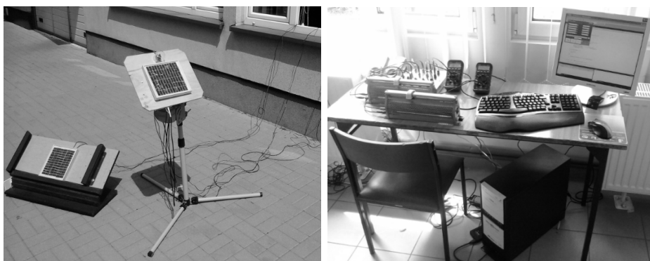
Fig. 1. A measurement stand consisting of a single – axis follow – up and fixed system for a photovoltaic modules
