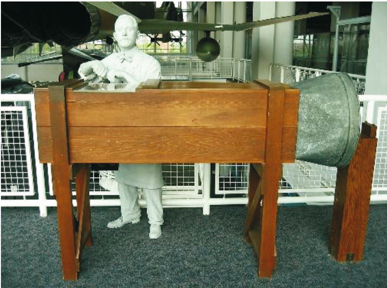
Fig. 3. Replica of the Wright Brothers' wind tunnel at the Virginia Air & Space Museum in Hampton, VA; source: photo by Erik Ax Dahl, licensed under the Creative Commons Attribution-Share Alike 2.5 Generic license 2006
