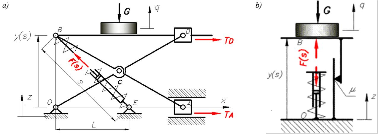
Fig. 1. Kinematic system of the seat suspension (a). Replacement model of the active seat suspension (b)
