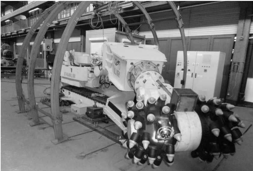
Fig. 1. R-130 boom-type roadheader (manufactured by Famur S.A.) on the test station at the Technology Hall of Faculty of Mining and Geology, Silesian University of Technology, Gliwice, Poland
