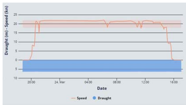
Figure 2. Ro-Pax ship’s “Victoria Seaways” speed distribution during the voyage Klaipeda – Kiel” (AIS information)
