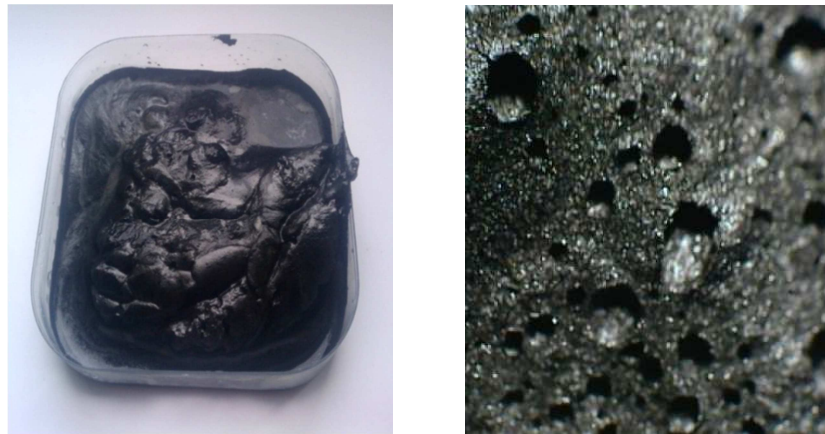
Fig. 12. Air-dried charcoal mass: a) of great porosity, b) comminuted with high-pressure water jet ( p= 250\text{MPa} )
