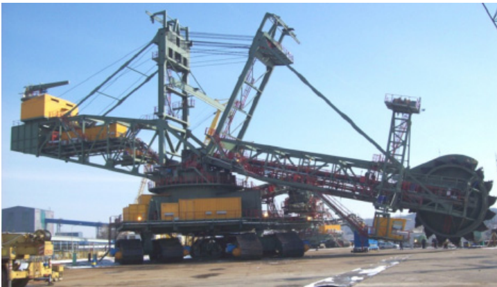
Fig. 1. BWE SchRs 1600: total mass (with mobile conveyor) 3345 t, mass of the superstructure 1233 t, theoretical capacity 6600 m 3 /h
