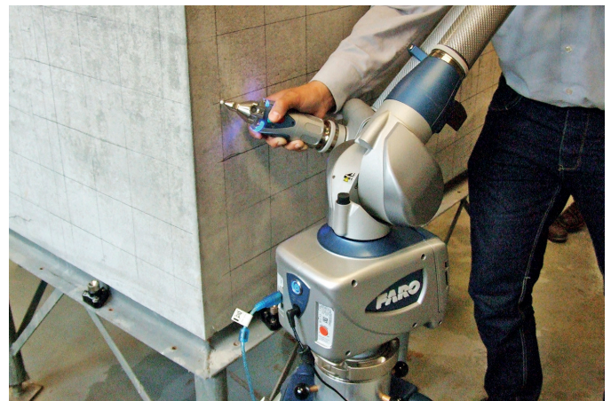
Fig. 6. Tank during measurements and visible reference points placed on a supporting steel frame
