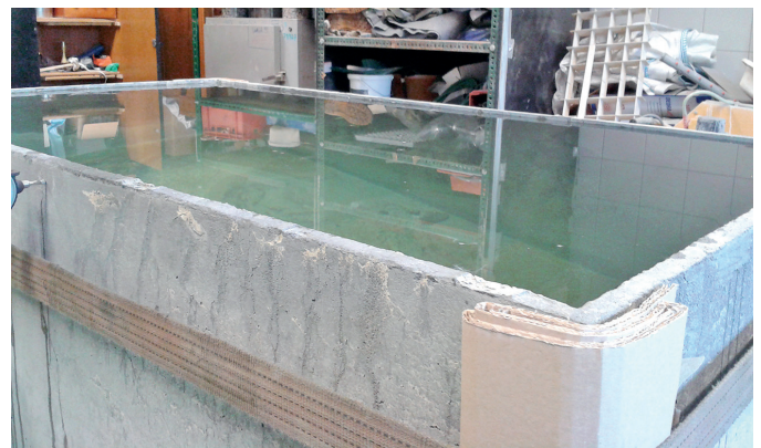
Fig. 5. Tank fully filled with water ready for deformation measurements
