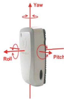
Fig. 6. Sensor's orientation angles - Ubisense
