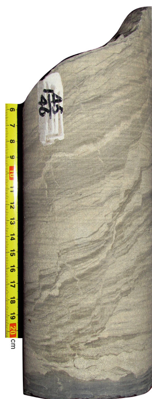
Fig. 3. Example of a core with a variety of small-scale soft-sediment deformation structures, including faults, bent laminae and intrusions of fluidised sediment. Core from well SP1, depth 1971.3 m.
