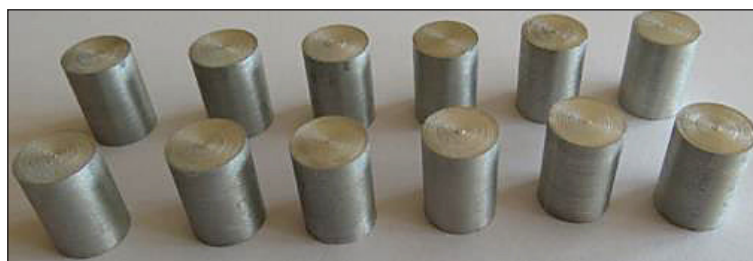
Figure 1. Example cylindrical samples used in the study ( \varnothing 20×30 mm)
