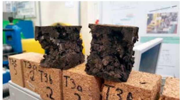
Figure 4. Tested samples of natural (dark) and agglomerated (light) cork
