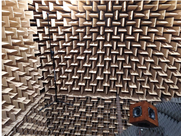
Figure 3. View of the hardware implementation of the acoustic field distribution test procedure.
