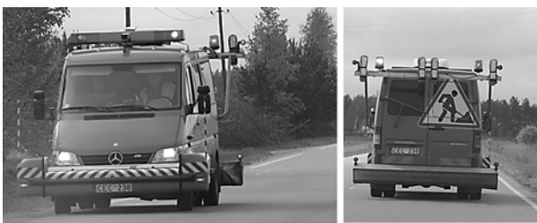
Fig. 2. Road surface testing laboratory RST 28
