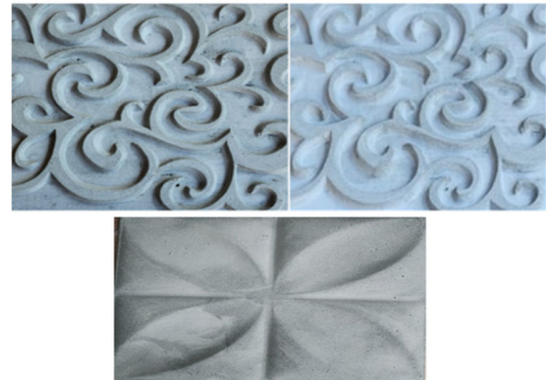
Fig. 4. The visual appearance of precast concrete wall panels with the addition of plastic powder and household ash as a partial replacement for sand and cement
