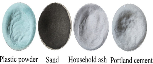
Fig. 1. Materials for preparing precast lightweight concrete wall panels
