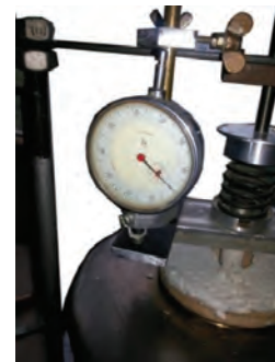
Fig. 3. Pressing device of the sintering setup
