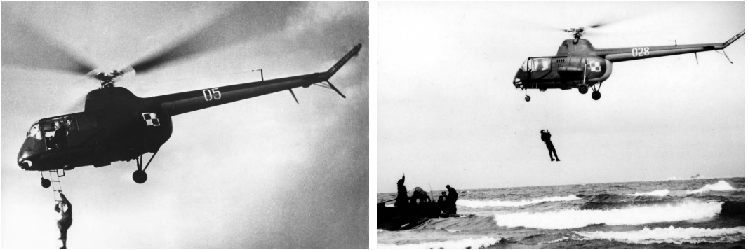
Fig. 8. Left – The SM-2 with a rope ladder, image – Karol Budniak’s collection, Right – The SM-2, even equipped with a winch, could only conduct rescue missions in the coastal zone, image – WAF.
