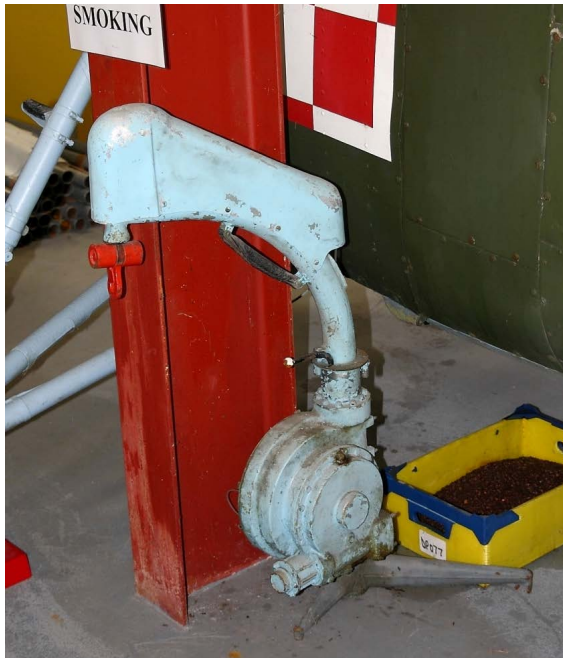
Fig. 9. Most likely the only surviving winch installed on the SM-2, currently located at the Helicopter Museum in Weston-super-Mare, Great Britain, image – Miłosz Rusiecki.
