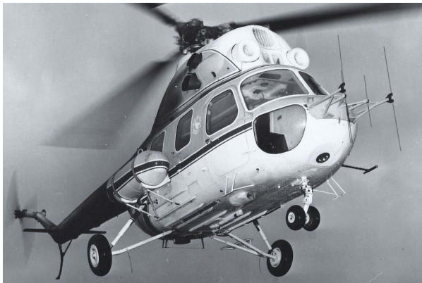
Fig. 6. Mi-2 “with a moustache”, equipped with the experimental emergency signal receiver / direction finder, designed by Krzysztof Kunachowicz, Eng. Image: Institute of Aviation via Ryszard Witkowski
