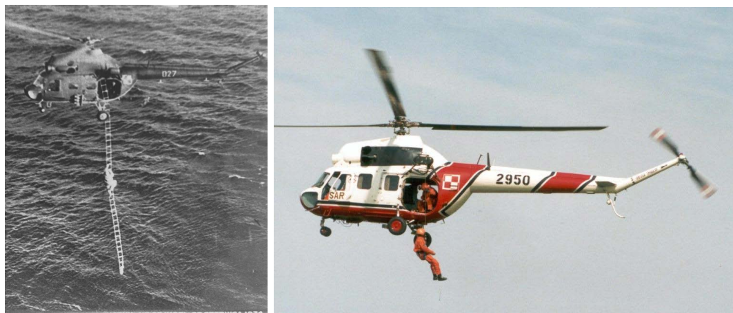
Fig. 10. Very good technical skills were required to climb aboard the helicopter using the rope ladder (left). It was impossible to use this method to lift an injured or an unconscious person. The image from the early stages of the helicopters' service life shows them sporting the original olive green liveries, the same as used on other military helicopters. Hydraulic, and then electric winches installed on the Mi-2RM made it possible to lower and hoist two people simultaneously – e.g. a rescuer and a victim (right). Images: WAF and Miłosz Rusiecki
