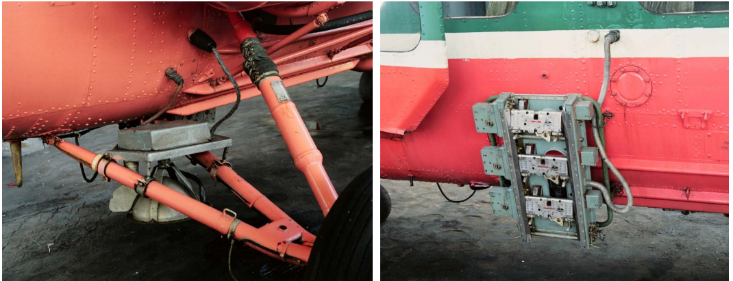
Fig. 4. Additional searchlights on the starboard side main landing gear strut, along with attachments for signaling bombs. Images: Miłosz Rusiecki
