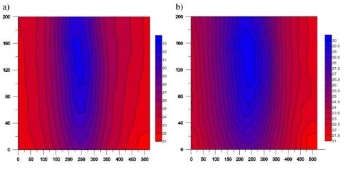
Fig. 2. The distribution of the radiation intensity radiant heater at a height of 1,9 m:a) the temprature field of heating suface in the non-rotary regime,b) the temprature field of heating suface in the rotary regime
