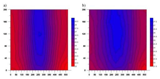
Fig. 3. The distribution of the radiation intensity radiant heater at a height of 2,8 m: a) the temprature field of heating suface in the non-rotary regime, b) the temprature field of heating suface in the rotary regime
