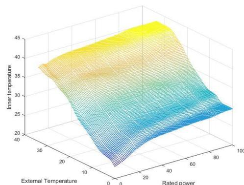
Fig. 3. The simulated data set for turbine T4, after the training of the ANN.
