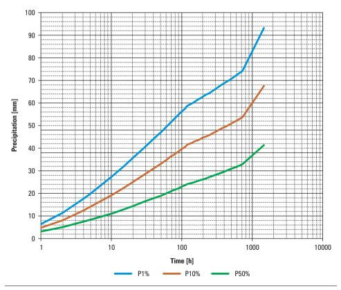
Fig. 1. Relationship between precipitation depth and duration for different probabilities of exceedance
