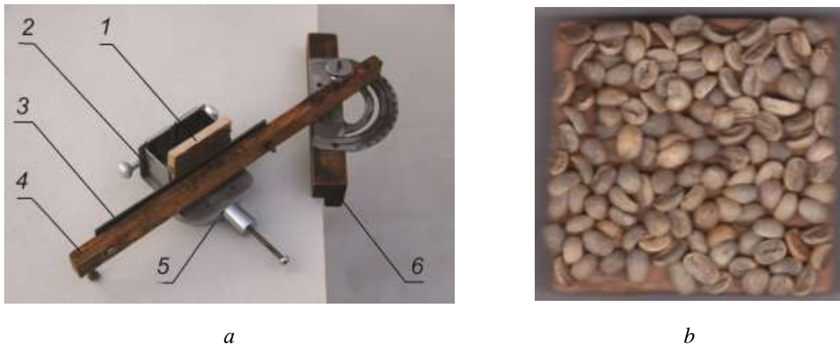
Fig. 1. Device for determination of sliding friction coefficient (a) and bar with coffee beans (b): 1 – bar of the research material, 2 – carriage 3 – sliding surface, 4 – ruler, 5 – automatic recorder 6 – guide block
